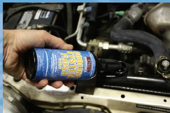
Step 6: Allow engine to run at least 15 minutes, up to 1 hour, after reaching normal operating temperature. The amount of running time will depend upon the condition of the coolant before starting the service. The more rust and calcium deposits you find, the longer the engine will have to be run at operating temperature.
