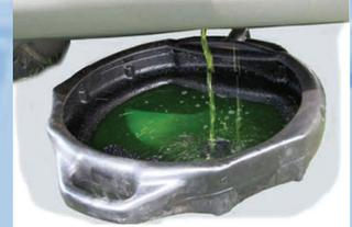
Step 9: Rinse cooling system with clear water until the fluid exiting the drain is clear.
