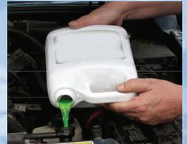
Step 12: Start engine and properly bleed cooling system per manufacturer's instructions.
