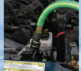
Step 10: Drain the now clean system and close the system drain plug.
