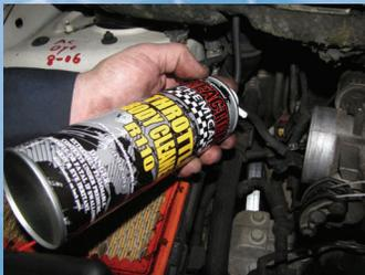
recommended procedure for opening the throttle plate. If the throttle is mechanically activated, the throttle may be opened by hand. Allow the cleaner to soak for 2-3 minutes. Reapply as necessary to complete cleaning. A soft rag may be used to aid in cleaning. A wire brush is not recommended to prevent damage to coated throttle body parts.
