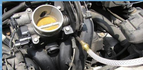
3. Attach the bottle of R100 Fuel System Cleaner to the R1425 Vacuum Applicator.
