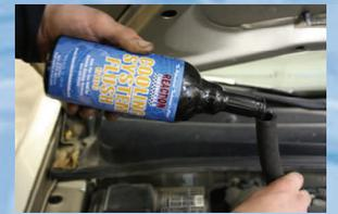
Step 10: Add hot water into the same temporary hose to completely fill the heater core. Allow to sit for 1 hour.
