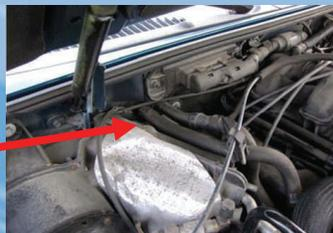
Step 5: Remove Heater Hose Clamps
