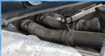
Step 6: Gently remove Heater Hoses-Take care not to crush the heater core nipples. It may be helpful to plan on replacing the heater hoses during this service. Catch any fluid that comes out of the core.
