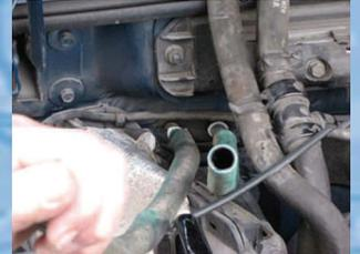
Step 9: Pour R106 Cooling System Flush into the heater core using one of the temporary hoses.
